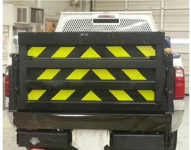
CHEVRON PATTERN ON LIFT GATE
